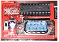
The interface board has a switch which sets the attached game-controller as **Left** or **Right**. The default position of the switch is **down** – **Left** joystick. The IJK-egoist interface works with the IJK-egopad but you can use it with any joystick from other 8-bit systems with DB-9 connector (C64, Atari etc.).
