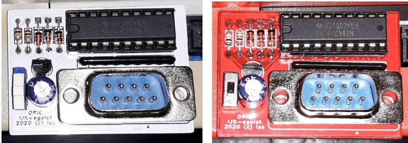
The interface board has a switch which sets the attached game-controller as **Left** or **Right**. The default position of the switch is **down** – **Left** joystick. The IJK-egoist interface works with the IJK-egopad but you can use it with any joystick from other 8-bit systems with DB-9 connector (C64, Atari etc.).
